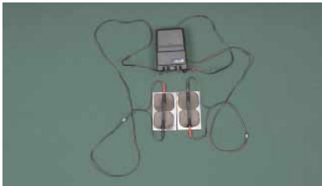
Figure 30-9 Transcutaneous Electrical Nerve Stimulation (TENS) Unit
